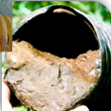
In order to prevent entry of sediments into drain pipes and blockage, pipes are wound by jacketing materials selected according to the characteristics of the soil where they will be installed and sold ready to use in recent years. Sand-gravel, pre-wound organic fibers, synthetic fibers, synthetic fabrics are widely used envelope materials. A practical application that will prevent penetration of plant roots into the pipes until now is to increase installation depth.
