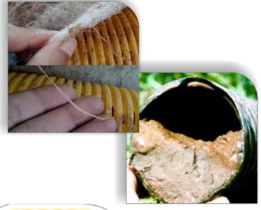
In order to prevent entry of sediments into drain pipes and blockage, pipes are wound by jacketing materials selected according to the characteristics of the soil where they will be installed and sold ready to use in recent years. Sand-gravel, pre-wound organic fibers, synthetic fibers, synthetic fabrics are widely used envelope materials. A practical application that will prevent penetration of plant roots into the pipes until now is to increase installation depth.
